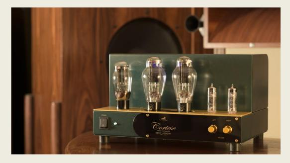
The Cortese is stereo single ended amplifier. Built to bring the qualities of his legendary reference products to a wider audience. Psvana 300B tubes are employed for 8 watts Class A output. Speakers of 90db sensitivity or higher are recommended.
